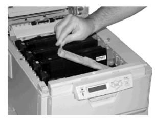
. Install the new toner cartridge in the image drum.
